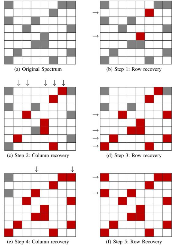
Fig. 1: An illustration of the “peeling” recovery process on an  $8 \times 8$  signal with 15 nonzero frequencies. In each step, the algorithm recovers all 1-sparse columns and rows (the recovered entries are depicted in red). The process converges after a few steps.
